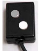
4) Attach the USB cable to the back of the digitizer and to USB port on your laptop. A red light should now appear on the top surface of the base. The USB port serves not only as the data connection, but also as the power source. Should your laptop not have power through the USB, an AC adapter is available.
