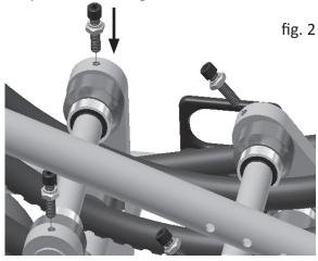
Hold screws in position with a 3/6" hex key wrench. Using a 7/6" wrench, tighten locking jam nut against frame (see fig. 3).
