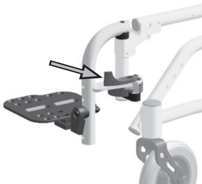
1. To swing away the hanger, place your finger tip on the inside of the hanger release lever.
