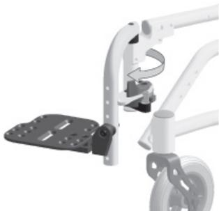
4. To attach the hanger, insert the pivot bushing into the frame receiver tube, at an angle as shown. Rotate the hanger inward until the latch snaps into place.
