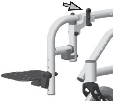
2. Pull back on the lever towards the chair. This will enable the hanger to pop-up and swing away for ease of transfer.
