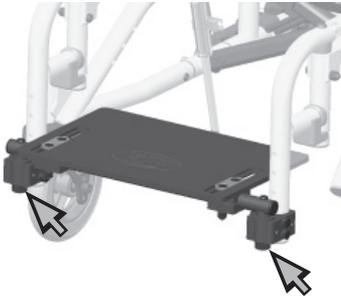
3. To attach the footboard after transfer, align the footboard fittings into the receivers. Turn the knobs on each side to tighten.
